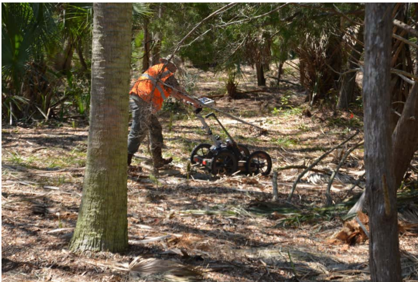
Figure 23. Photos of geophysical work. At the top is the Geonics EM-61. Below is the MALA Geosciences GPR system in use.
