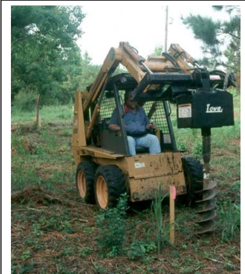
Figure 13. Using a "Bobcat" to conduct the auger testing on the site.
