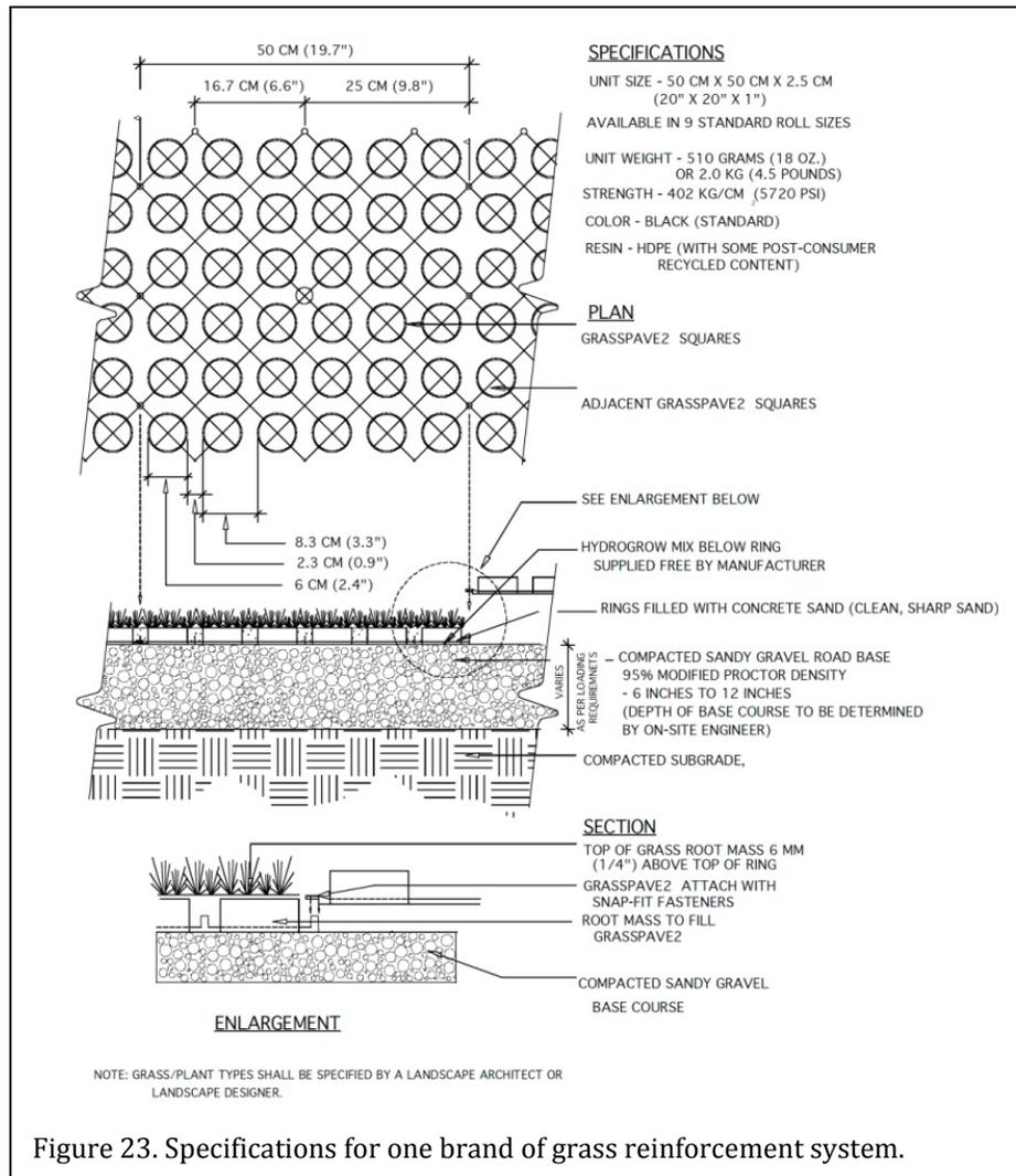
Figure 23. Specifications for one brand of grass reinforcement system.
