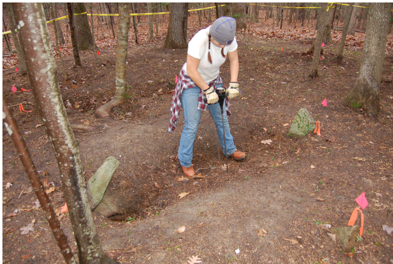
Figure 14. “Calibrating” the penetrometer by examining the compaction in a suspected grave.
