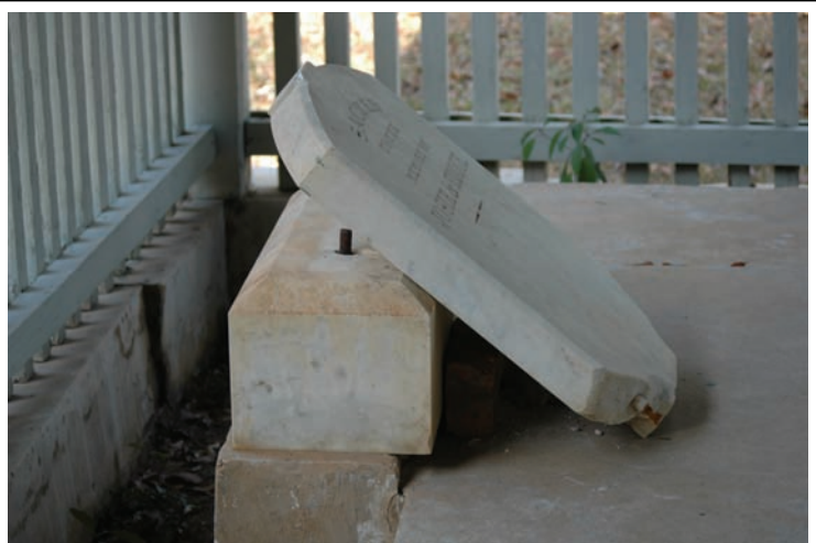
Figure 31. Stone with damage from ferrous pins. Note the loss to the lower corners of the monument.
