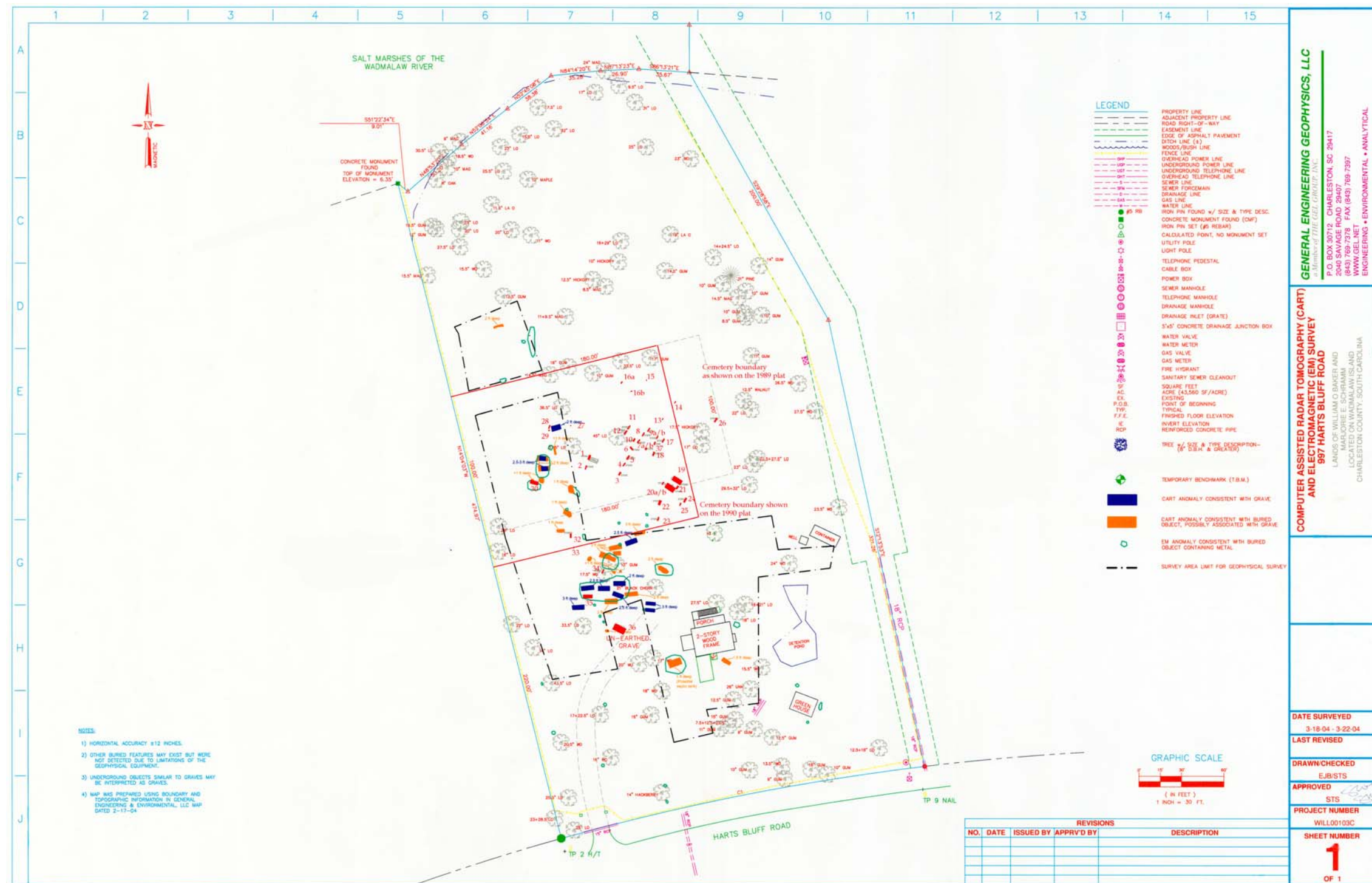
Figure 8. Basemap prepared by General Engineering Geophysics showing areas of ground penetrating radar and electromagnetic study. The only modifications made to this plan are the highlighting and numbering of existing graves and the addition of the cemetery boundaries portrayed by the 1990 plat.
