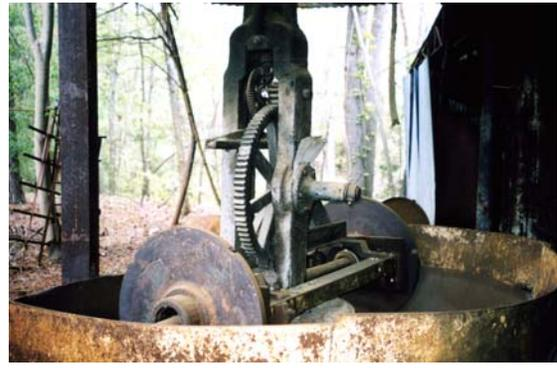
Chaser mill showing pan and two heavy iron wheels.
