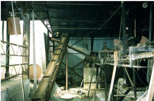
Conveyor for ground clay moving it up to the pug mill.
