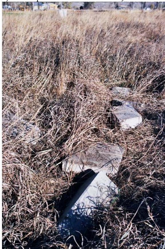
Cast iron fence posts broken off at ground level (note clean break at same location on both)
