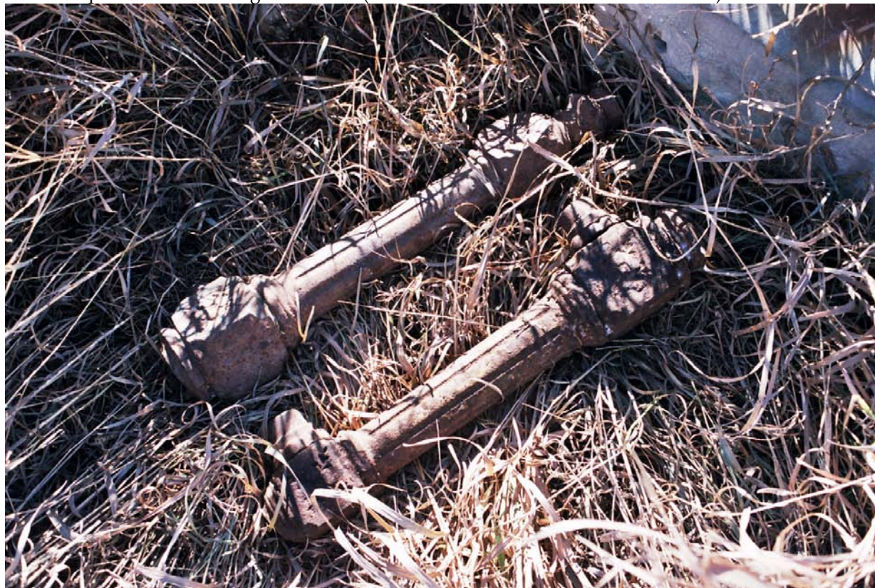
Cast iron fence posts broken off at ground level (note clean break at same location on both)
