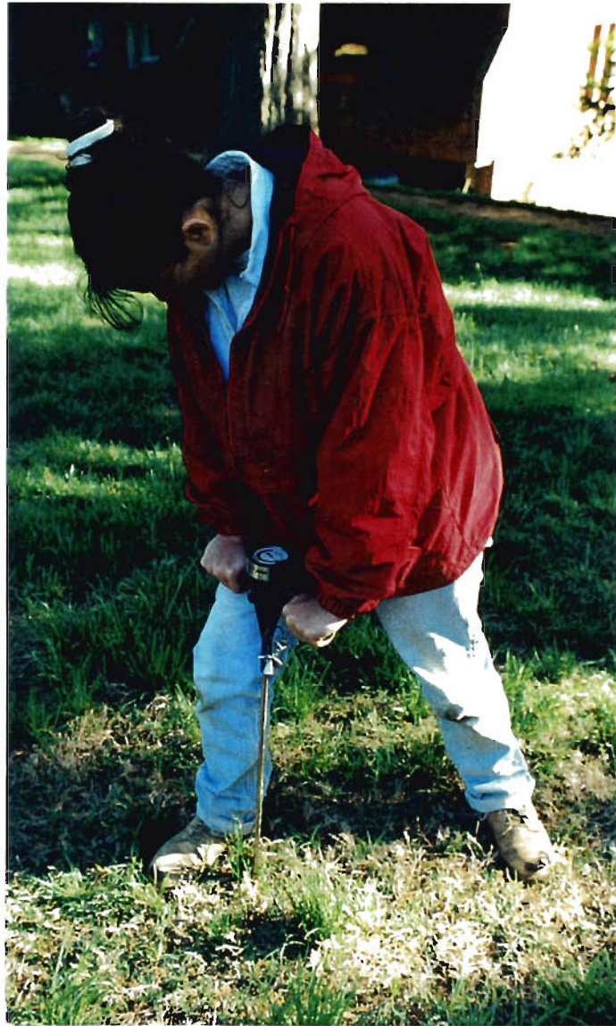
Figure 4. Using a penetrometer to determine grave locations.
