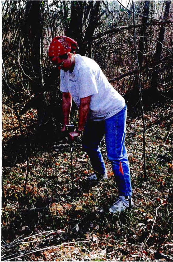
Figure 3. Use of a penetrometer to identify grave locations on the Pye property at the Kings Cemetery.
